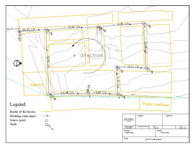
Figure 3. The initial water flow and direction
