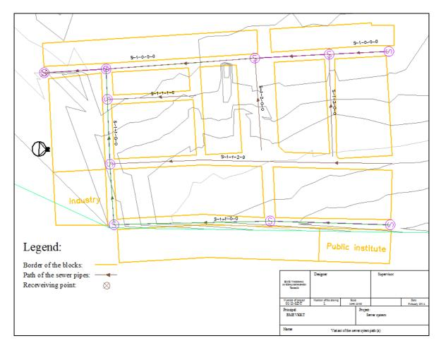
Figure 4. Path variant of the sewer sytem
