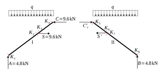
Positive side is set to the bottom of each oblique member. Calculations from the left and right hand side on either member I or II are performed on the basis of sign conventions shown below:
