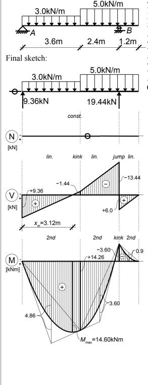
Solution Resultants:  $R_1 = 3.0 \cdot 3.6 = 10.8 \text{ kN}, R_2 = 5.0 \cdot 3.6 = 18 \text{ kN}$ Reactions:  $\sum M_i^{(A)} := -10.8 \cdot 1.8 - 18 \cdot 5.4 + B \cdot 6.0 = 0$   $\Rightarrow B = 19.44 \text{ kN}(\uparrow)$   $\sum M_i^{(B)} : 10.8 \cdot 4.2 + 18 \cdot 0.6 - A_2 \cdot 6.0 = 0$   $\Rightarrow A_2 = 9.36 \text{ kN}(\uparrow)$   $\sum F_{ix} : A_x = 0$ Check:  $\sum F_{iz} : 3.0 \cdot 3.6 + 5.0 \cdot 3.6 - 9.36 - 19.44 = 0$
