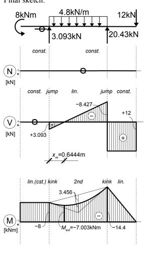
Normal forces could arise from horizontal forces; in their absence the diagram is constant with a zero value.
