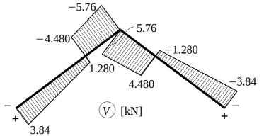
$K_3$  is calculated from the right. Reaction C leftwards and distributed load on the right of the cross section result in a negative and positive shear, respectively:
