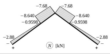
Calculation in  $K_{7}$  is done from the right. Reaction *B* upwards and distributed load down wards result in compression and tension, respectively:
