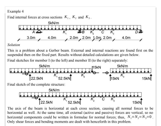
section  $K_1$  from left based on member I:  $V_1 = 22.5 - 5.7 = -12.5 \text{ kN}$  $M_1 = 22.5 \cdot 4 - (5 \cdot 7) \cdot 3.5 = -32.5 \,\text{kNm}$  $V_1 = 22.5 - 5.7 = -12.5 \text{ kN}$  $M_1 = 22.5 \cdot 4 - (5 \cdot 7) \cdot 3.5 = -32.5 \,\mathrm{kNm}$
