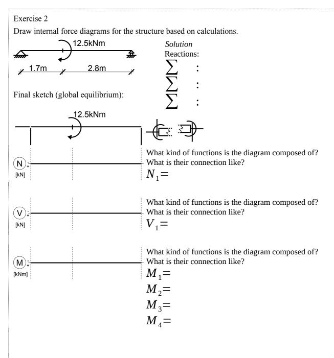
Check the existence and sense of jumps and kinks, as well as whether or not some lines are parallel to each other.
