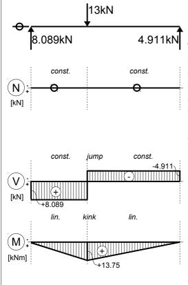
Solution Support reactions should still be found first:  $\sum M_i^{(A)}:-13\cdot1.7+B\cdot4.5=0 \rightarrow B=4.911 \text{ kN}(\uparrow)$   $\sum M_i^{(B)}:13\cdot2.8-A_z\cdot4.5=0 \rightarrow A_z=8.089 \text{ kN}(\uparrow)$   $\sum F_{ix}:A_x=0 \text{ kN}$ Check:  $\sum F_{iz}:13-4.911-8.089=0$
