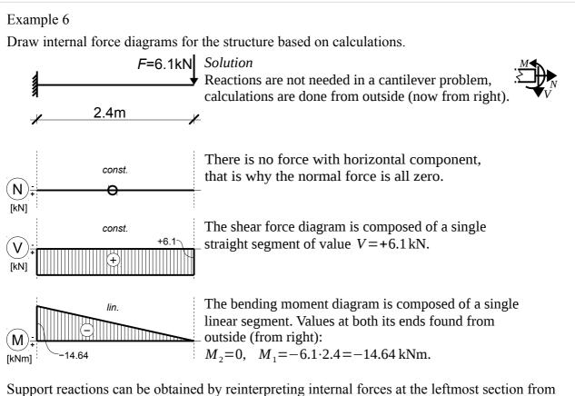
Support reactions can be obtained by reinterpreting internal forces at the leftmost section from left:  $V \blacktriangle_{M}$
