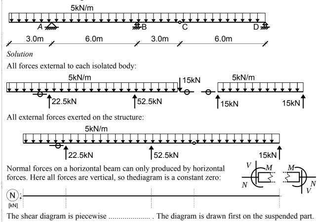
The arrangement of forces resembles that of a simply supported beam with a constant distributed load. The shear force values needed to draw a linear segment are as follows:
