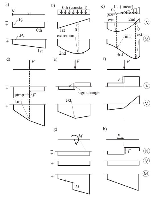
The relationship between the load and the bending moment diagram can be verified in a quite ingenuous way by imagining the load to be exerted on a rubber string. The shape of the string corresponds then to the bending moment diagram: unloaded segments remain straight, concentrated and distributed forces cause kinks and curvatures in it, respectively.
