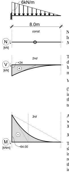
Solution Reactions are not needed in a cantilever problem. Internal forces are found proceeding from the free end to the support, calculations are done from outside (now from right).
