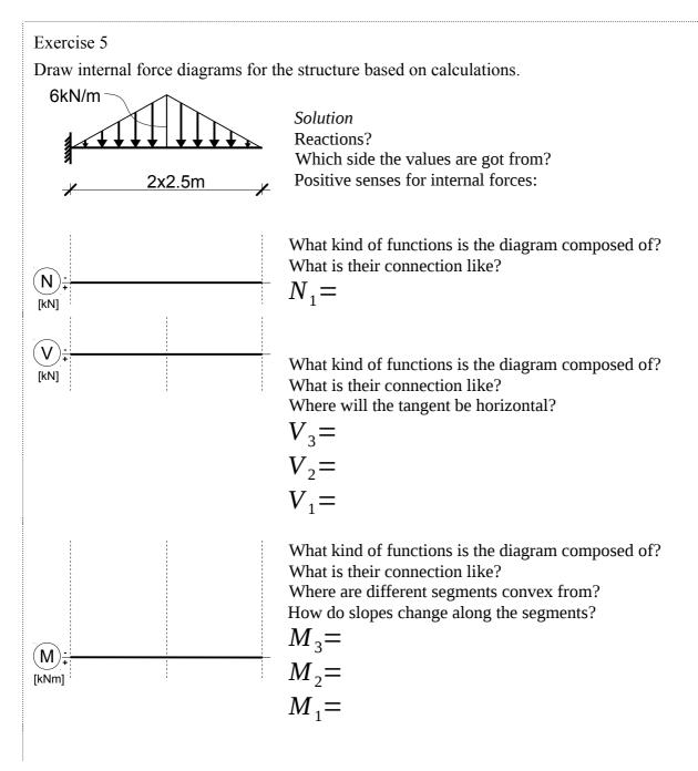
Draw internal force diagrams for the structure based on calculations.
