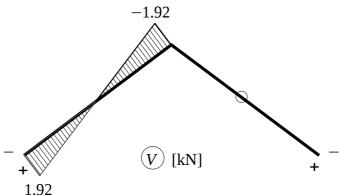
$K_2$  is easier to be calculated from the right. Both reactions  $C_2$  upwards and  $C_x$  leftwards cause a negative shear:
