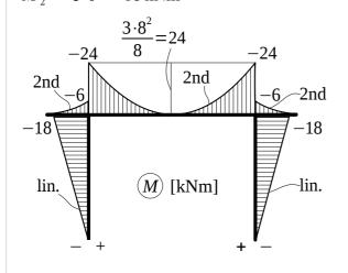
Similarly, if the moment in  $K_9$  is calculated from below, the reaction component  $B_x$  (inwards) results in tension on the right hand side of the column and is therefore negative:
