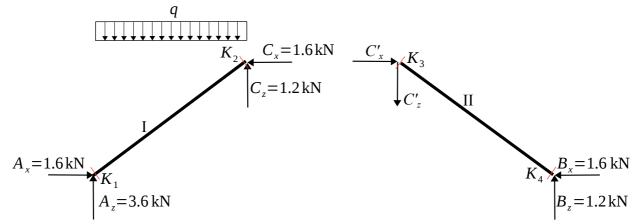
Positive side is set to the bottom of each oblique member. Calculations from the left and right hand side on either member I or II are performed on the basis of sign conventions shown below:
