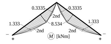
Note that symmetric loading (including active and passive forces exerted on the structure) on symmetric structures yield always symmetric normal and bending moment diagrams and an anti-symmetric shear force diagram. This last term refers to the property that ordinates in symmetric position are of equal magnitude but opposite sign.
