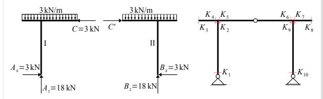
Positive side of horizontal segments of the frame is set to the bottom; thus, for convenience, the inner side is considered positive in both vertical segments. Sign conventions for the left hand side vertical segment (calculation from the bottom side), for the horizontal segment (from left and from right), as well as for the right hand side vertical segment (from the bottom) are as follows:
