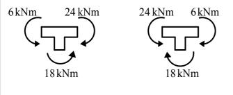
Finally, nodal moment equilibrium of each bifurcation should be checked. Accounting for tensile sides of all cross sections, arrows of bending moments are drawn to the nodes and their sums are calculated.
