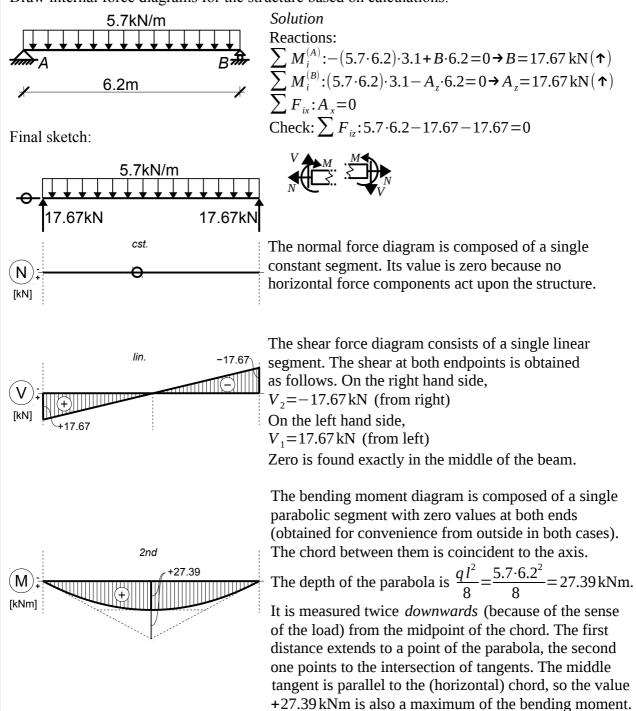
*About the M diagram*: There are zero values at both ends (in the absence of any torque there). The load is directed downwards, therefore the depth of parabola is measured downwards as well.
