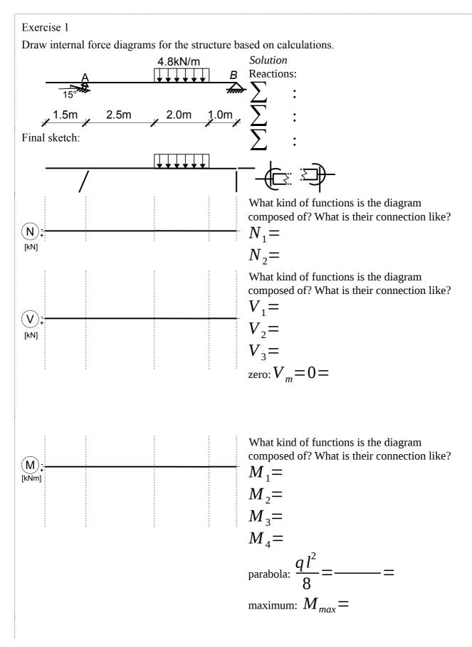
Draw internal force diagrams for the structure based on calculations.
