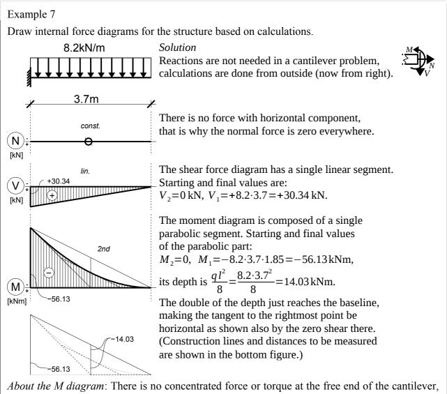
*About the M diagram*: There is no concentrated force or torque at the free end of the cantilever, hence the parabolic segment starts from zero and with a zero slope there. The parabola is convex from below because the load is directed downwards.
