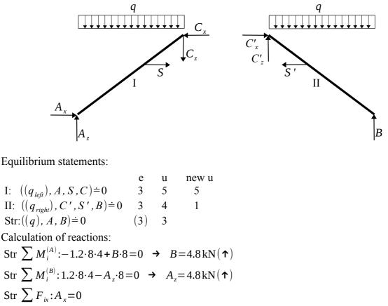
$$\begin{split} \text{II} & \sum M_i^{(C)} := -1.2 \cdot 4 \cdot 2 + 4.8 \cdot 4 - S' \cdot 1 = 0 \quad \Rightarrow \quad S' = 9.6 \text{ kN}(t) \\ \text{II} & \sum F_{ix} : C'_x - 9.6 = 0 \quad \Rightarrow \quad C'_x = 9.6 \text{ kN}(\Rightarrow) \\ \text{II} & \sum F_{iz} : 1.2 \cdot 4 - C'_z - 4.8 = 0 \quad \Rightarrow \quad C'_z = 0 \text{ kN} \end{split}$$
