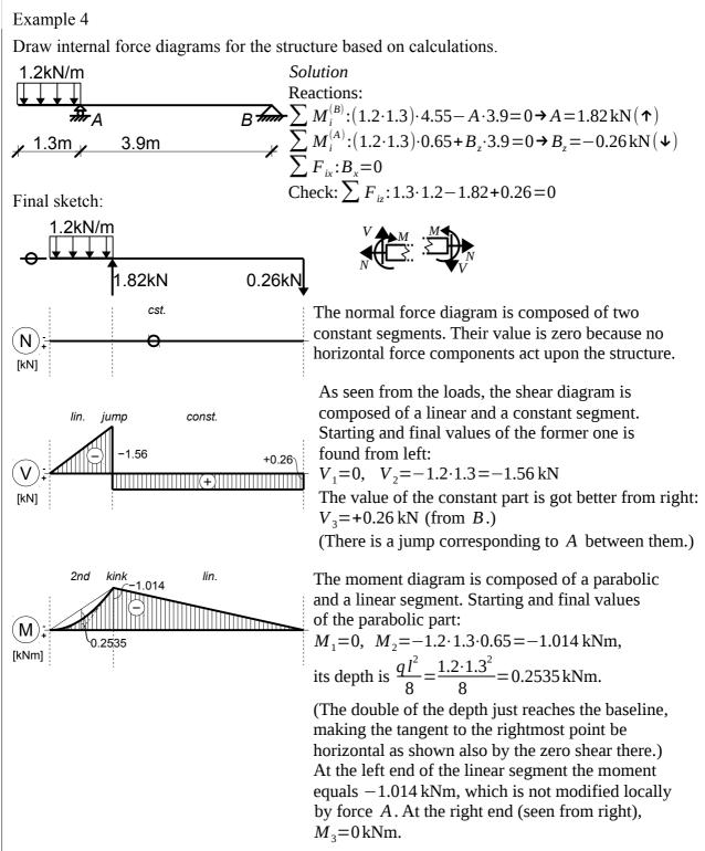
*About the M diagram*: There is no concentrated force or torque at the end of the overhang, hence the (parabolic) segment starts from zero and with a zero slope there. The parabola is convex from below because the load is directed downwards. Due to the support reaction, the diagram has a kink at the right hand side of parabolic segments and continues linearly to the rightmost point. The right endpoint of the diagram is zero because of the absence of any concentrated torque again.
