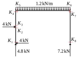
The solution starts by finding all reaction components; they are sketched in the figure to the left (the method of their calculation has already been demonstrated in Example 1 of Lecture 11).
