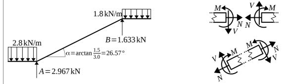
The normal force diagram is composed of three constant segments (two horizontal and an inclined one). On horizontal parts, any normal force is due to horizontal components. Since all external forces are vertical, those are all zero:  $N_1 = N_3 = 0$  kNm. If a value on the inclined part is calculated from (bottom) left, normal resolutions of reaction A and distributed load (of intensity 2.8 kN/m) should be considered:
