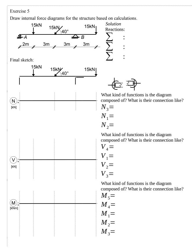
Draw internal force diagrams for the structure based on calculations.
