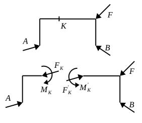
The component of the force vector parallel to the axis of the bar is called *normal force* and denoted by N (as a reference to that the axial force is parallel to the normal direction of the cross section). A component of the force vector that lies within the plane of cross section is called *shear(ing force)*
