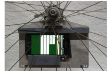
Figure 4: A Samsung Galaxy S2 as a wheel sensor at radius r_s = 9.5 cm in a bicycle wheel of radius r_w = 35 cm for data logging.
