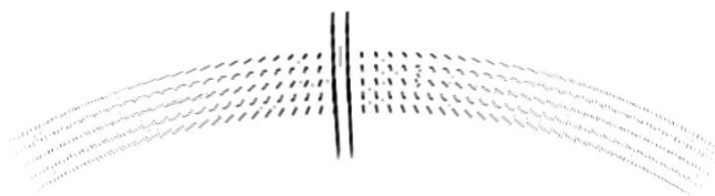
Figure 3.16: Displacement vectors when the load is applied to the middle span
