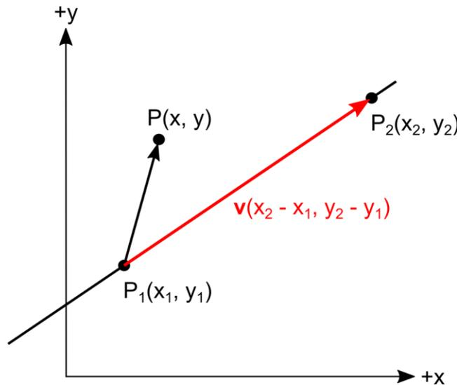
Figure 6. Equation of a line using two points.
