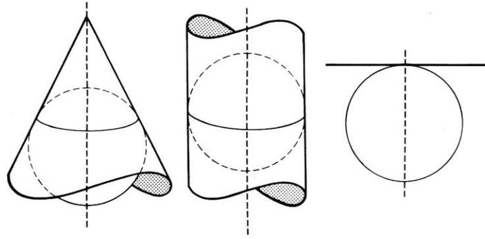
Figure 1. The developable projection surfaces of the conic (left), the cylindrical (center) and the azimuthal (right) projections.
