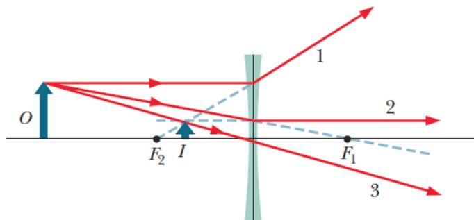
Figure 2. Ray tracing with a diverging lens.
