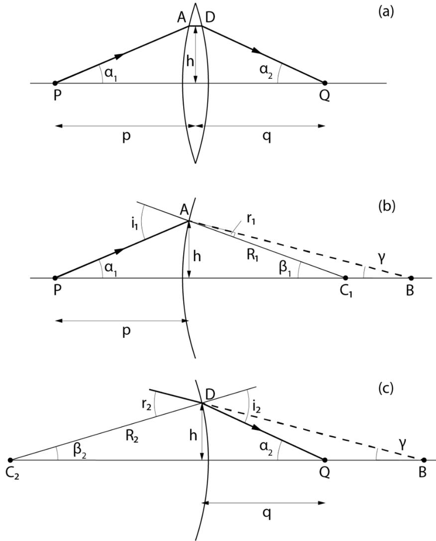
Figure 3. Derivation of the lens maker's equation.
