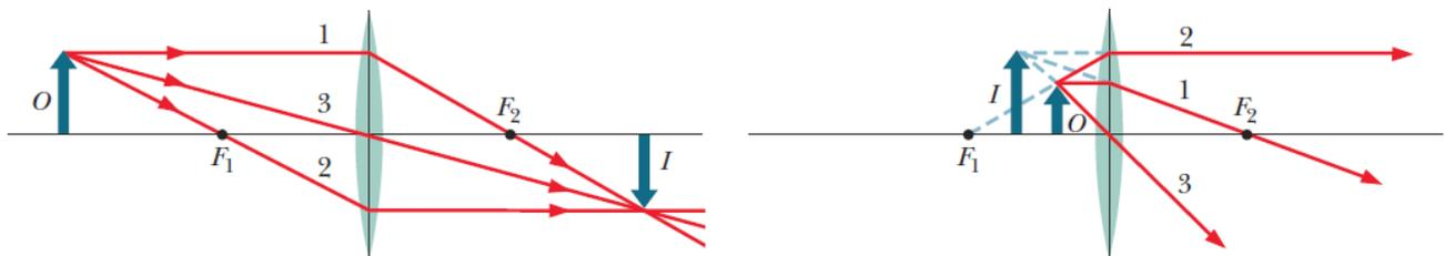
Figure 1. Ray tracing with a converging lens.
