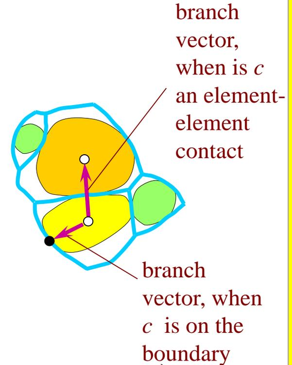
$$\bar{\sigma}_{ij} = \frac{1}{V} \sum_{(L)} \left( \sum_{(Lc \in S^L)} v_i^{Lc} F_j^{Lc} \right) = \frac{1}{V} \left( \sum_{(c \text{ inside})} (v_i^{Lc} - v_i^{Kc}) F_j^{Lc} + \sum_{(c \text{ boundary})} v_i^{Lc} F_j^{Lc} \right) =$$
