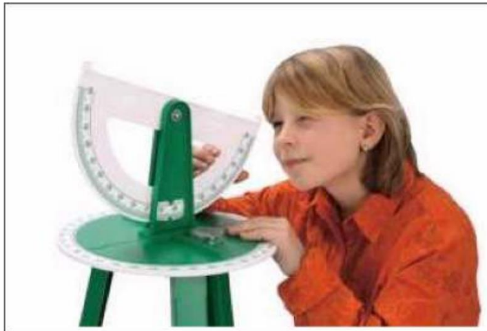
Theodolite in its most basic form
