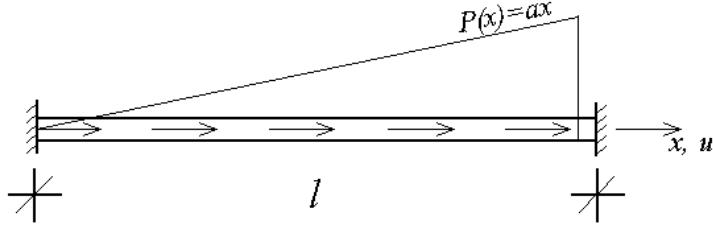
This is an axially loaded bar of which the potential energy is:
