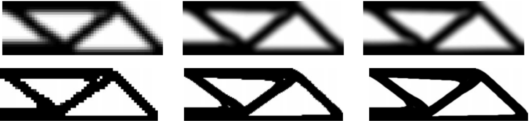
Optimal layouts using the same filtering radius r_{min} and finer meshes: density filter vs. HS projection filter
