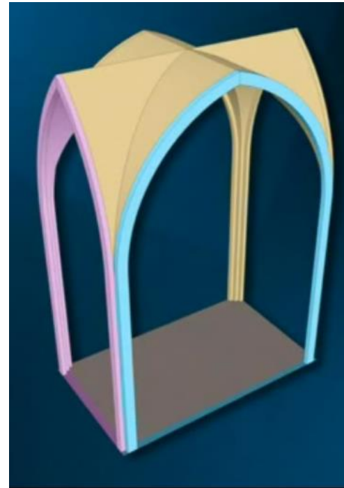
one bay of the vault
