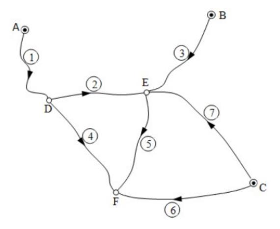
We measured the height differences along levelling lines 1-7. We also have three benchmarks (points with known elevations) in the area, A, B and C. Our goal is to calculate the elevation of points D, E and F using all the available measurements. As we have 7 measurements and 3 uknown elevations (m > n in matrix **A**), we can only find an optimal solution when the sum of the squared errors of the elevations are minimalized. (The arrows in the figure show the direction of rise in the lines.)
